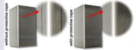
Picture left shows typical marks of a fold, right image without calling for use of bending foils
