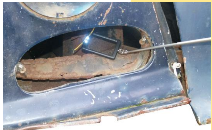
Backlighting and testing of narrow and difficult to access places
