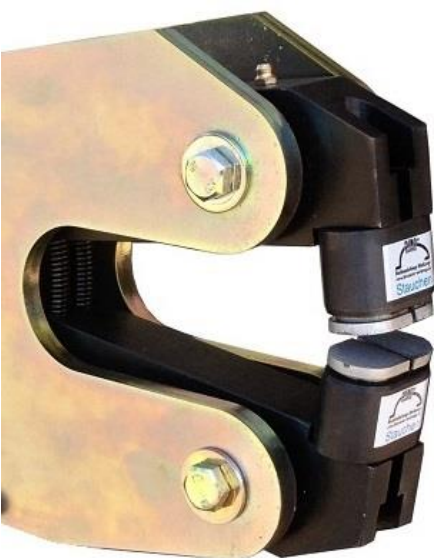
Installation of oval shrinking-stretching tools
